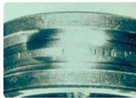
Stage 3: The debris is over-rolled; real surface spalling develops.
